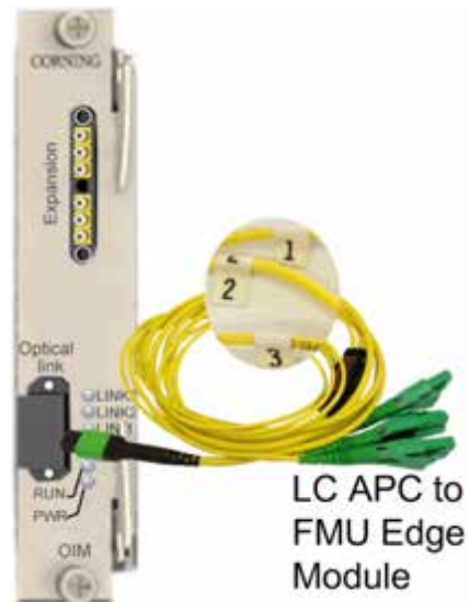
Figure 9: OIM Fiber Connections
