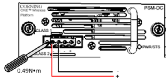
Figure 8. Example of DC CLASS1 Wiring
