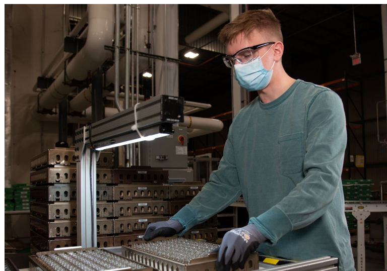
A Corning Pharmaceutical Technologies employee loads vials in preparation for the ion exchange process.
