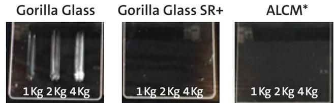
Figure 1 - Gorilla Glass SR+ scratch performance vs. other materials (150 grit garnet sandpaper scratch test, 1 cycle under 1, 2 and 4 kg loads)
