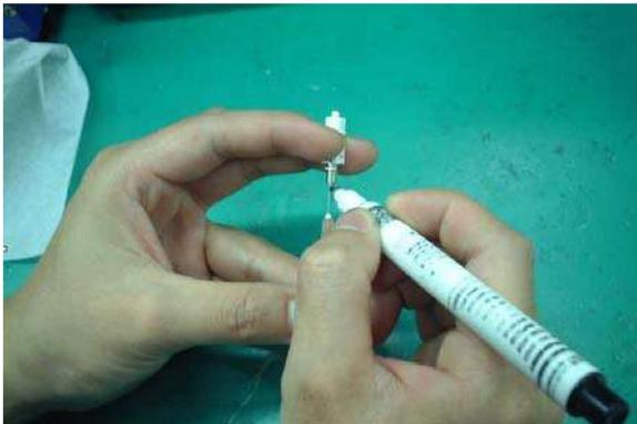
**Step 4** Insert the syringe tip into the rear of the connector until it bottoms with the ceramic ferrule. Place a mark with marking pen, the mark just below the connector. See Fig. 5.
