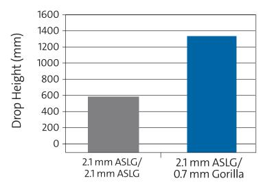
Gorilla hybrid laminates can be more than 2x impact resistant to blunt or sharp stones, resulting in fewer severe cracks.
