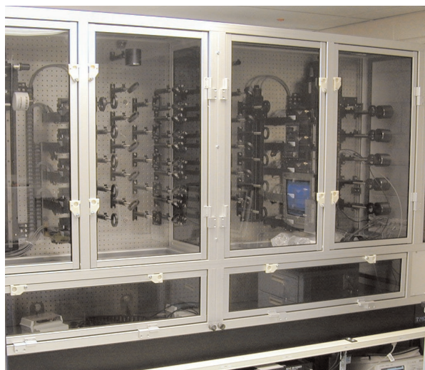
ArF Laser Damage System at Corning
