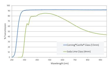
Corning Gorilla Glass exhibits higher transmission performance and superior optical clarity in the visible range.
