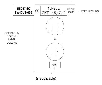
Note: GFCI labeling is required on all receptacles that are protected by such devices. In the event that "normal" receptacles are series fed from GFCI receptacles, each receptacle in series with the actual GFCI
