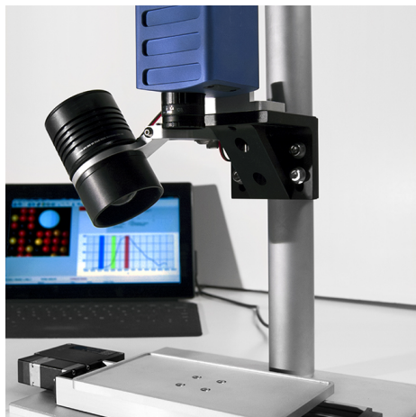
Hyperspectral Application Development Kit containing a motorized linear-transition stage.
