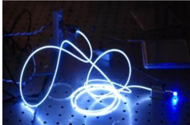
Figure 11. White light emanating from an LDF fiber powered with a blue 445 nm laser diode. The color conversion of blue light to white light is done using a Ce-YAG phosphor doped into the coating of the fiber.
