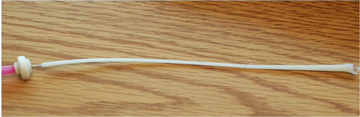
Figure 3. This is a picture of a photocured polymer that was cured inside a 4mm i.d. opaque tube. An LDF fiber was placed into the center of the tube filled with a photocurable polymer. The LDF was powered with a 355nm laser. After irradiation, the polymer was completely cured around the fiber.
