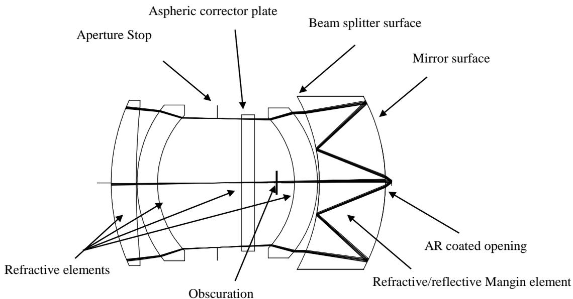
Figure 3. Major components in a small field Newtonian objective
