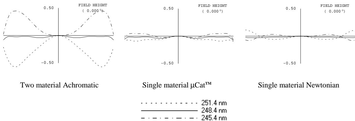
Figure 16. Comparing 0.6 NA design amounts of Spherochromatic optical path difference (OPD) for broad bandwidth
