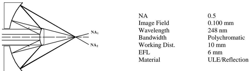
Figure 10. Long working distance two mirror reflective objective
