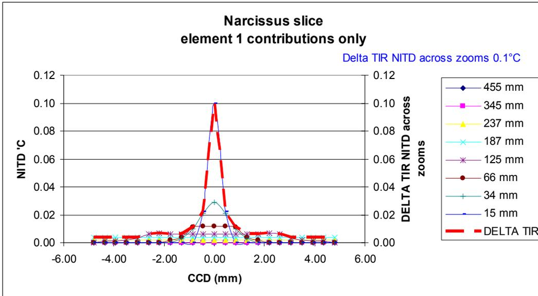
Figure 11. The Narcissus effects of the front element are shown here. Element 1 contributes 1/3 of the total narcissus difference across the zoom range.
