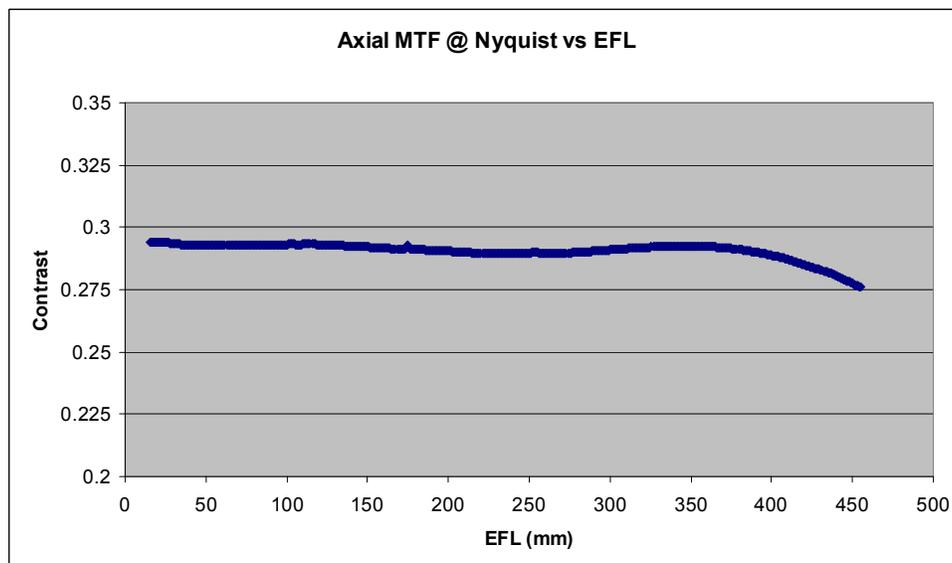
Figure 9. The small discontinuity of focus is hardly visible in this plot showing the axial MTF value at Nyquist across the zoom range.
