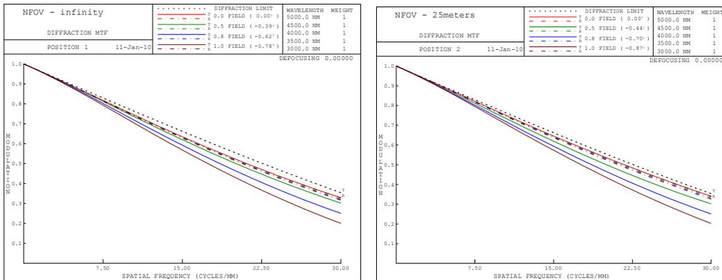
Figure 16. The nominal MTF curves for an object at infinity are shown on the left, with the corresponding MTF for an object at 25 meters is on the right.
