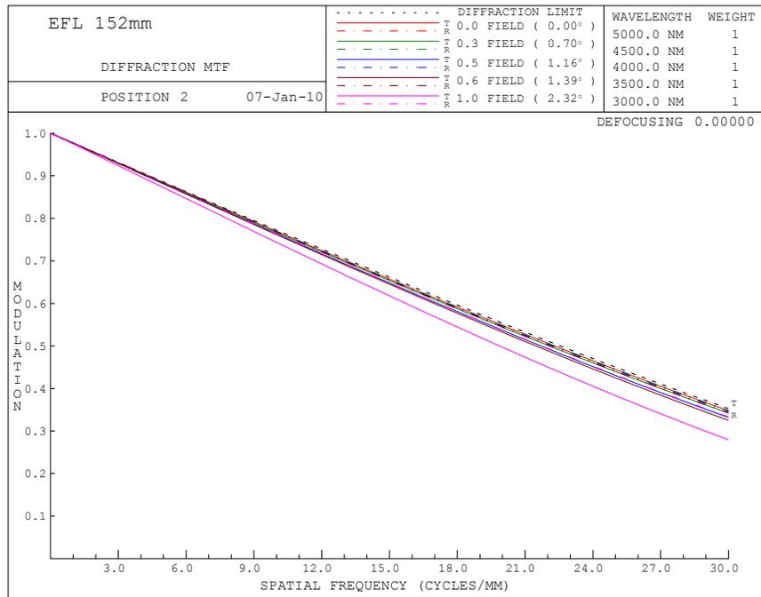
Figure 3. A typical MFOV MTF is shown out to Nyquist of the designed camera. Through most of the zoom range, the system is diffraction limited.
