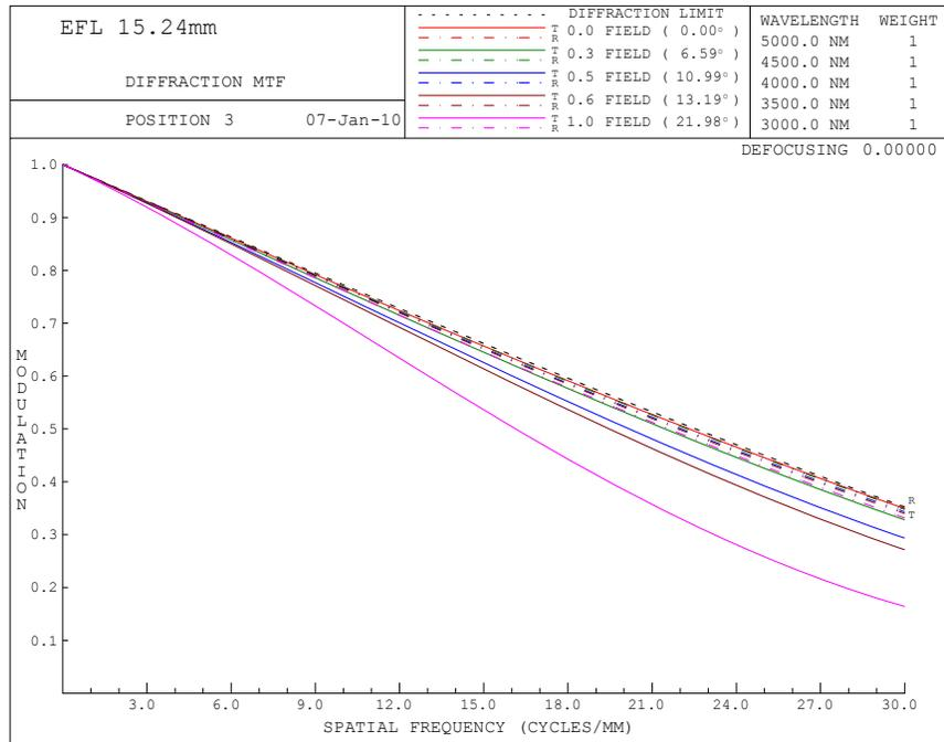
Figure 4. The WFOV MTF is shown out to Nyquist of the designed camera. There is some drop in performance only at the very corner of the FOV.
