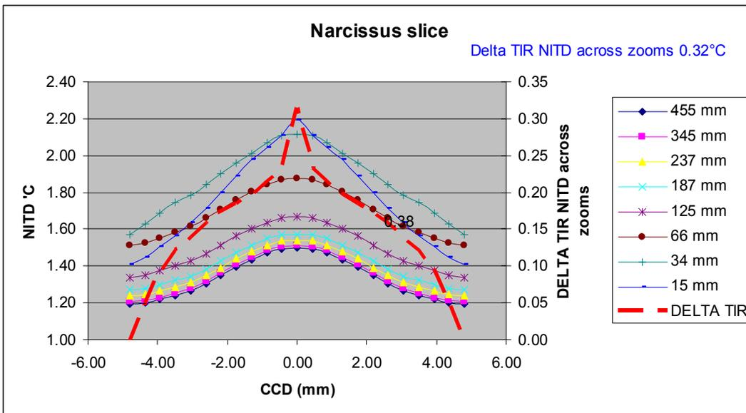
Figure 12. This graph illustrates the Narcissus affects at different focal lengths. Multiple calibrations can be taken to reduce the effect.
