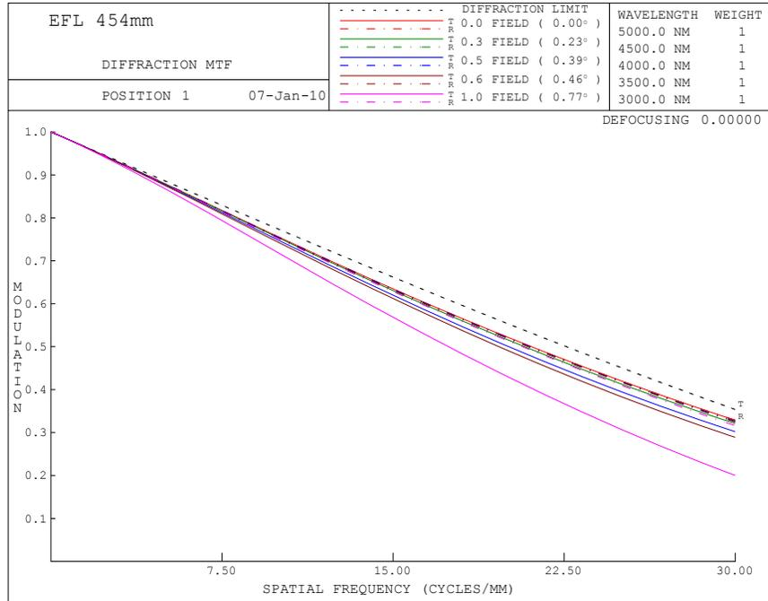
Figure 2. The NFOV MTF is shown out to Nyquist of the designed camera. It is close to the diffraction limit for the entire field.
