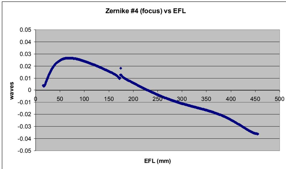
Figure 8. The small discontinuity of focus can be seen from this plot. The amount of defocus is negligible.
