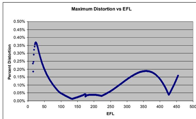
Figure 5. The distortion of the system is low through the entire zoom range.
