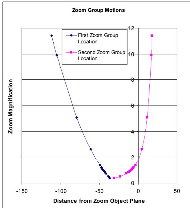
Figure 6. The zoom paths of the system are smooth. We used extra care in the region where the zoom magnification was 1X.
