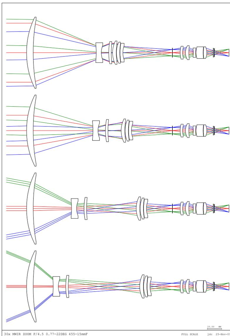
Figure 1. The layout shows the smooth path of the zoom groups throughout the range. It also shows that the WFOV is not limited by any glass to glass collisions.
