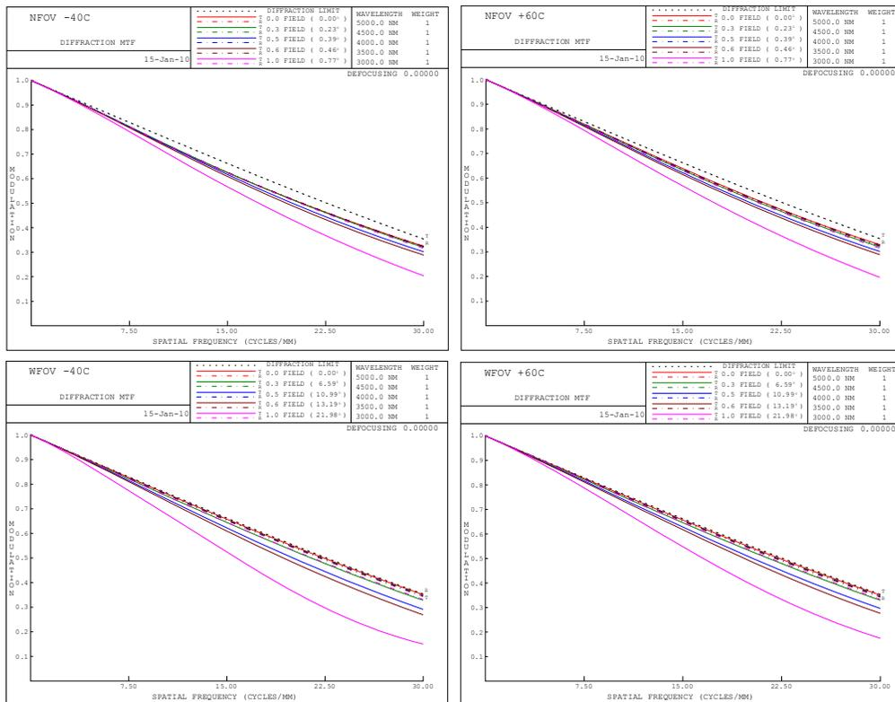
Figure 13. The MTF plots of the NFOV and WFOV at both temperature extremes show no loss of performance after application of active compensation.
