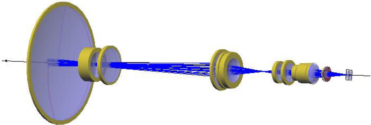
Figure 10. The front element is the largest contributor to narcissus. The single bounce ghost is shown here.
