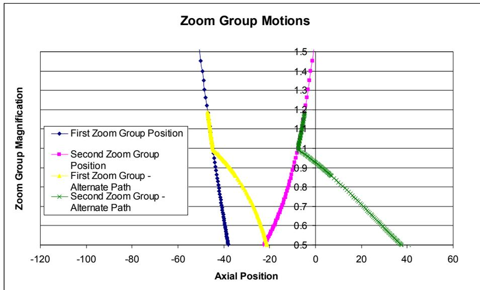
Figure 7. The “alternative” zoom paths deviate from the smooth designed path at the 1X zoom magnification location.
