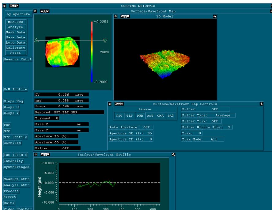
Figure 4. Data and interferogram of an off-axis reflective asphere after compensation.
