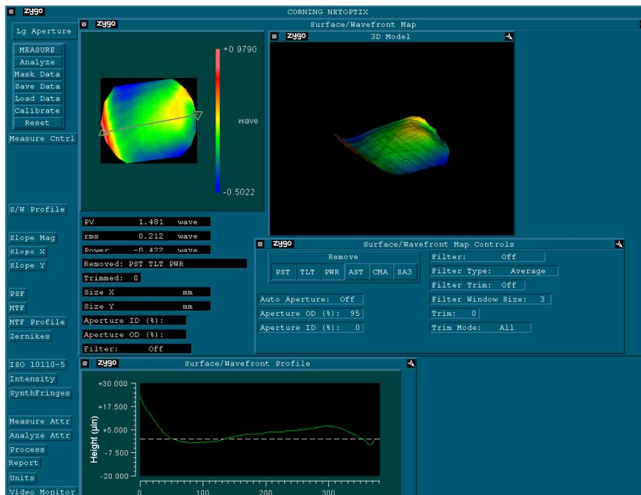
Figure 3. Data and interferogram of an off-axis reflective asphere before compensation.
