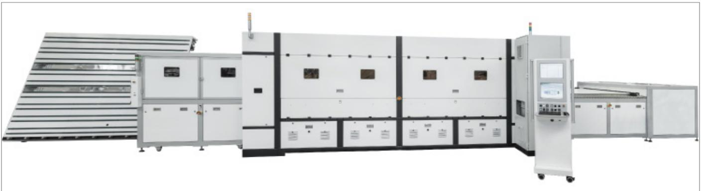
Using ultra-short laser pulses, the CLT 80G cuts by material disassociation rather than ablation. The result is a very low surface roughness, increased as-cut edge strength and faster throughput. The Corning Laser Technologies process enables cutting fully strengthened glass, Corning® Gorilla® glass, un-strengthened glass, as well as other transparent glass and crystalline materials.
