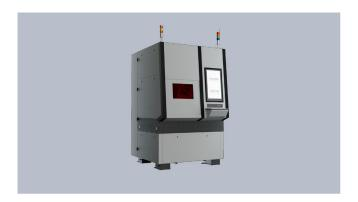
The CLT's laser dicing process is a two-step approach of modification and separation: the modification of glass - wafers is done by CLT's well-established laser process while the separation can be realized by automated breaking on stretch tape. The results are increased processing speed, improved accuracy and minimal particle generation as well as increased utilization of wafers with small dies by more than 20%.
