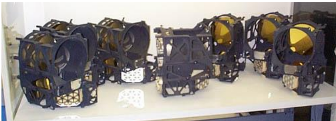
Figure 6 Offner-like “Snap Together” Reflective Assembly
