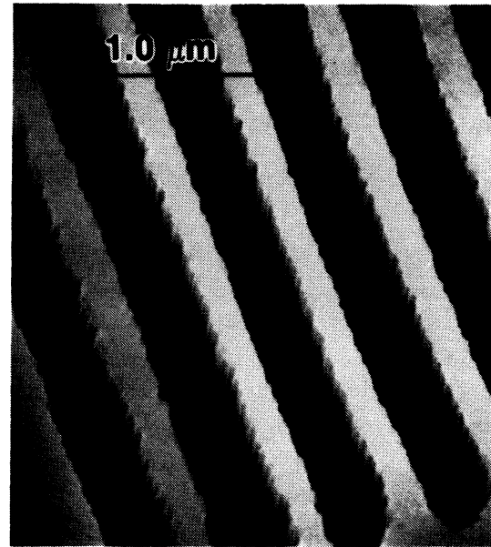
Fig.8b. 0.2 \mu\text{m} lines and spaces transferred into the silicon wafer.
