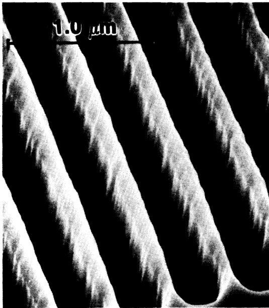
Fig.8a. SEM photo of 0.2 \mu\text{m} lines and spaces transferred from the imaging layer into the bottom resist layer.
