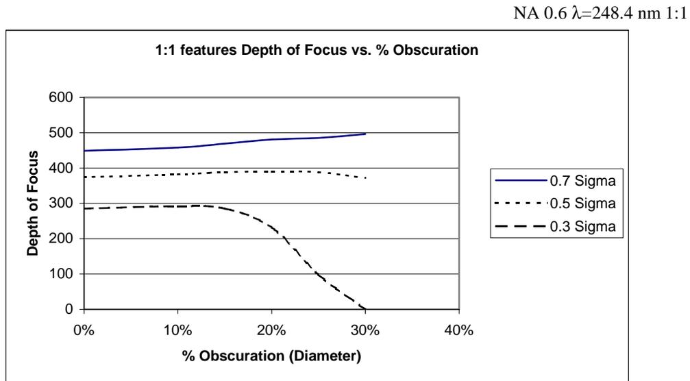
Figure 14. Effect that central obscuration has on partial coherent depth of focus for different pupil fill
