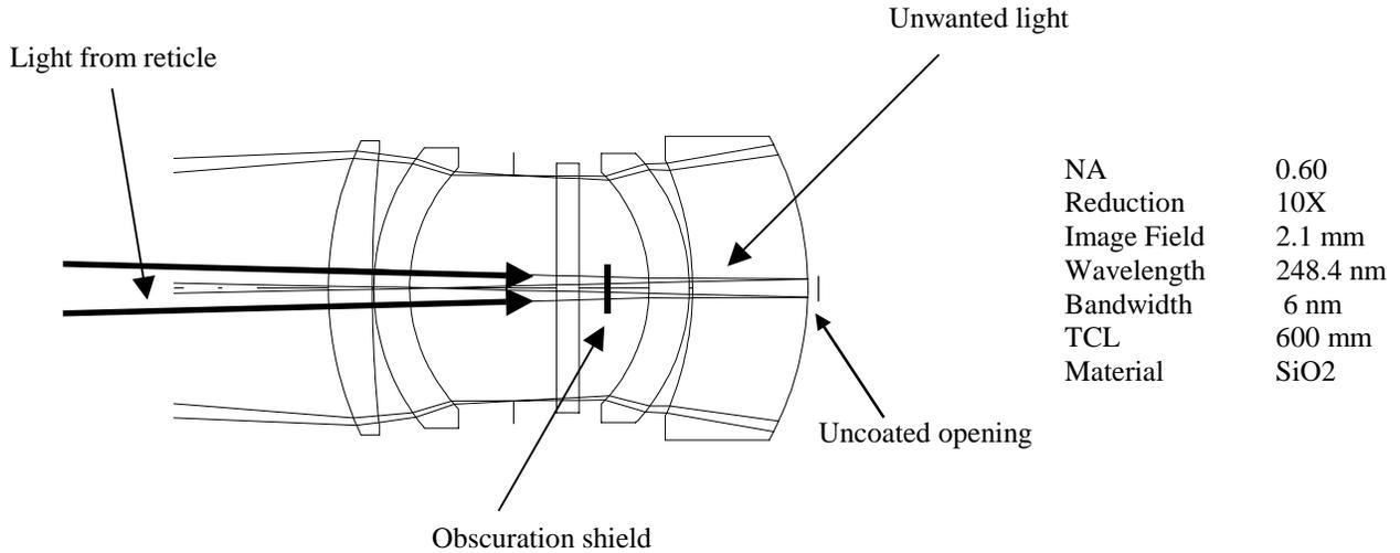
Figure 4. Central obscuration shields image plane from unwanted light passing directly through opening
