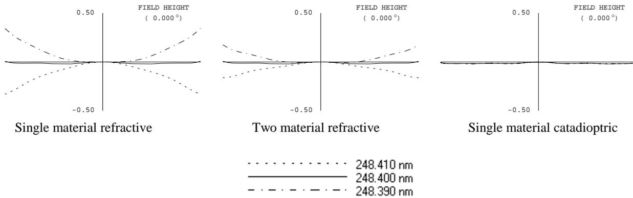
Figure 15. Comparing 0.75 NA design amounts of chromatic optical path difference (OPD) for narrow bandwidth
