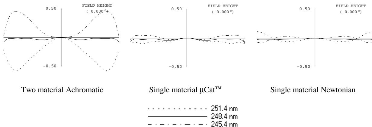
Figure 16. Comparing 0.6 NA design amounts of Spherochromatic optical path difference (OPD) for broad bandwidth
