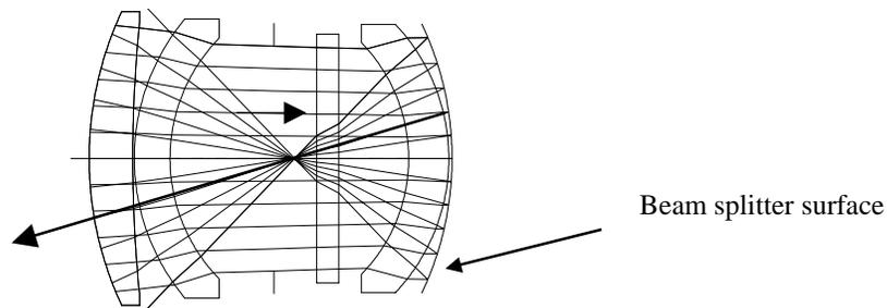
Figure 5. Reflected light off the beamsplitter travels away from the image plane
