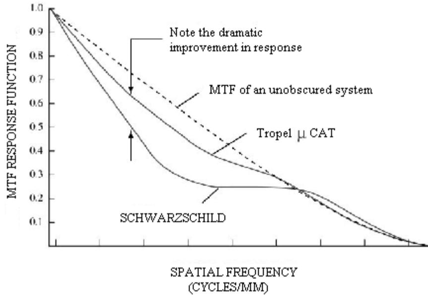
Figure 13. Best focus MTF Curve showing effect of central obscuration on the response function
