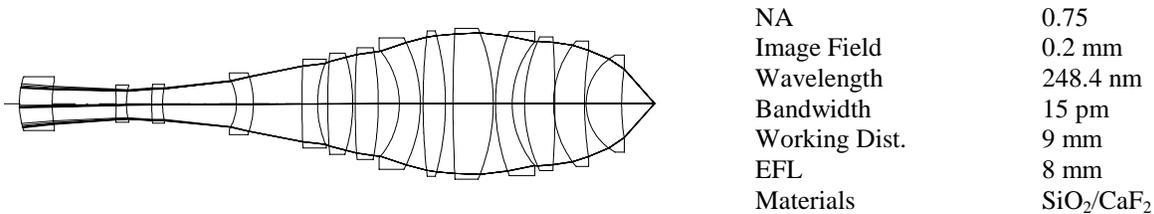
Figure 9. 0.75 NA long working distance objective for reticle inspection at 248 nm
