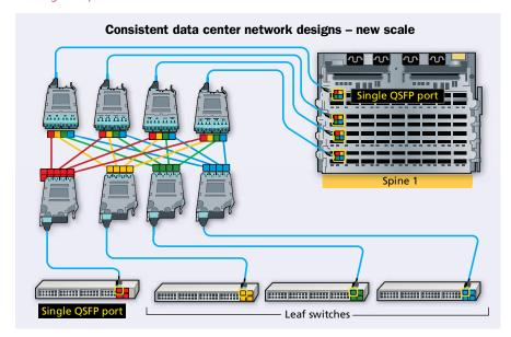
While this is not the most elegant approach, this setup shows a 10-Gbit crossconnect using 8-fiber breakout modules. By making an LC patch connection between respective leaf and spine switches, a user can break out all 40-Gbit ports and distribute them over four different line cards. This approach maintains redundancy, because if a line card is lost, only 25 percent of bandwidth is lost.
