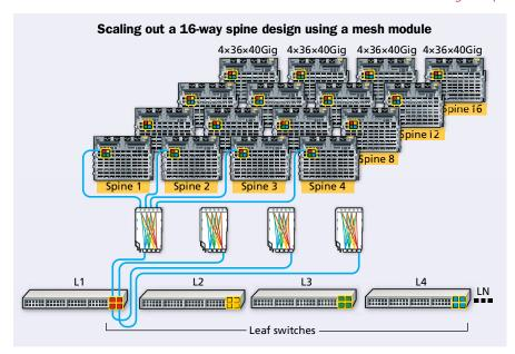
Using the mesh-module scenario, we can go beyond a two-way spine and even beyond a four-way spine, to a 16-way spine as depicted here. Implementing this approach, a user does lose the line-card-level redundancy and switching efficiency; however the user gains more redundancy by distributing risk over the 16-way spine. With this type of implementation, it is worth investing in fabric modules, because this scenario includes different leaf switches on different line cards in the same chassis.
