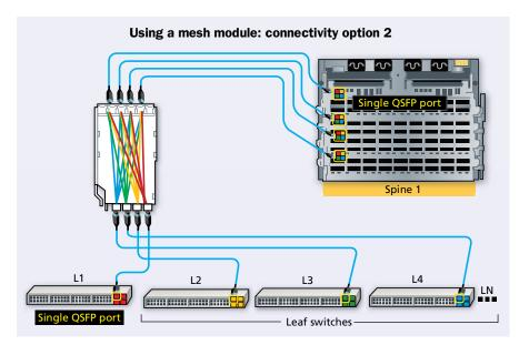
In this setup a mesh module is connected to the spine on one side and to the leaf on the other side. Spine-side ports connect to individual line cards on the spine switch. Every time the user connects a leaf switch on the leaf side, that port is automatically broken out and shuffled across the spine ports on the mesh module—which are already connected to separate line cards. No LC-to-LC patching is required.
