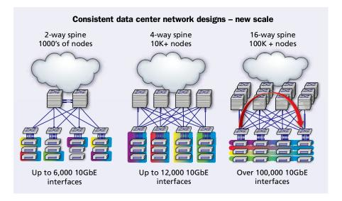
In a spine-and-leaf network fabric, leaf switches control the flow of traffic between servers and spine switches forward traffic along optimal paths between leaf switches. An architecture known as 16-way spine can scale to support more than 100,000, 10-Gbit Ethernet hosts.
