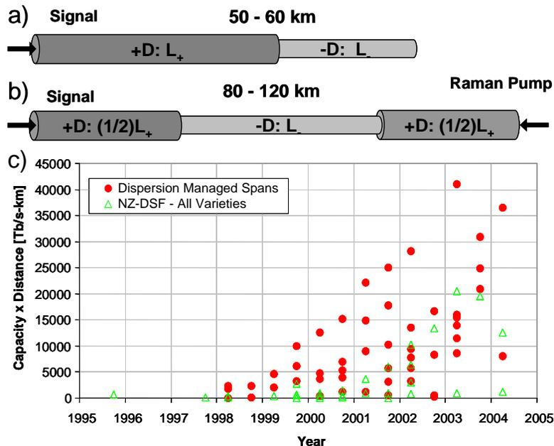
**Figure 1.** Configurations for submarine (a) and terrestrial DMF (b) and capacity reach product for DMF and other NZDSFs including medium dispersion fiber reported in OFC and ECOC hero experiments (c).
