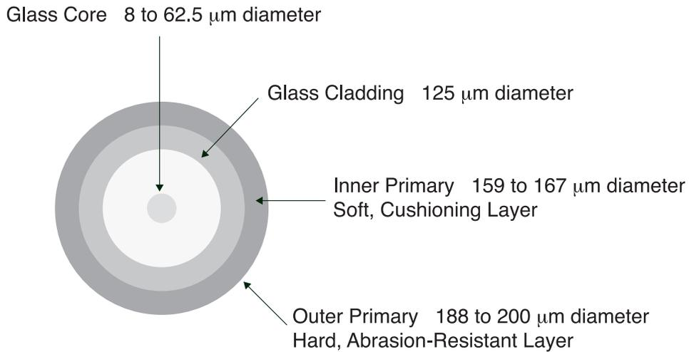
Figure 2. Schematic of a Reduced Fiber Diameter Dual Layer Coating Design
