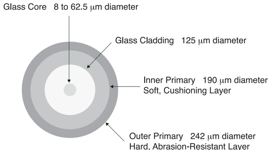
Figure 1. Schematic of a Dual Layer Coating Design
