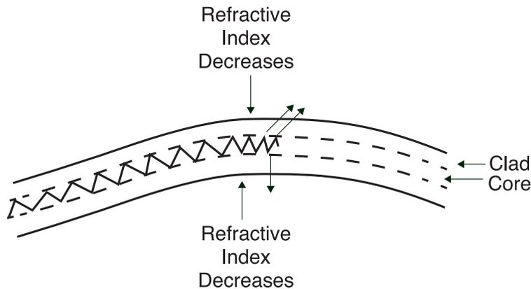
Figure 3. Fiber Microbending Due to Mechanical Testing
