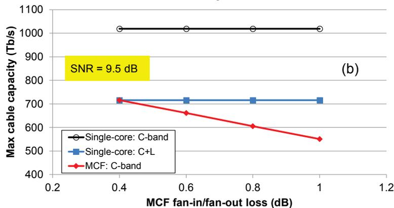
Fig. 3: Maximum cable capacity as a function of MCF fan-in/fan-out loss in repeaters.
