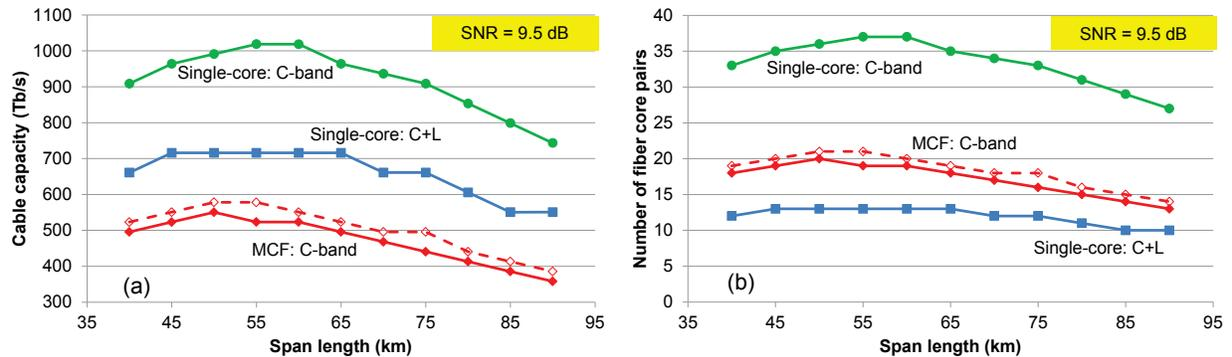
Fig. 1: a) Cable capacity vs. span length. b) Number of fiber core pairs supported vs. span length. SNR target = 9.5 dB.
