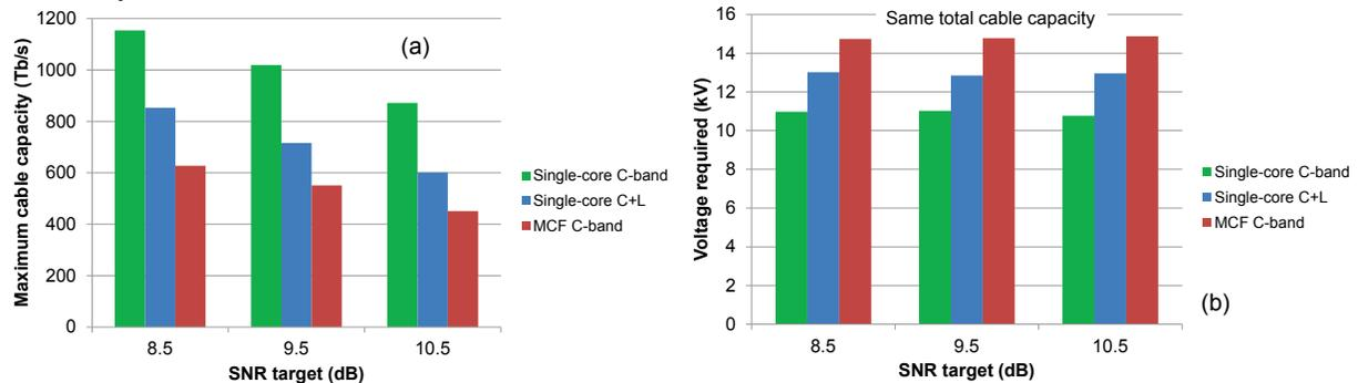
Fig. 2: a) Maximum cable capacity vs. SNR target for voltage up to 15 kV. b) Required voltage with equal cable capacities with 60 km spans for each SNR target value.
