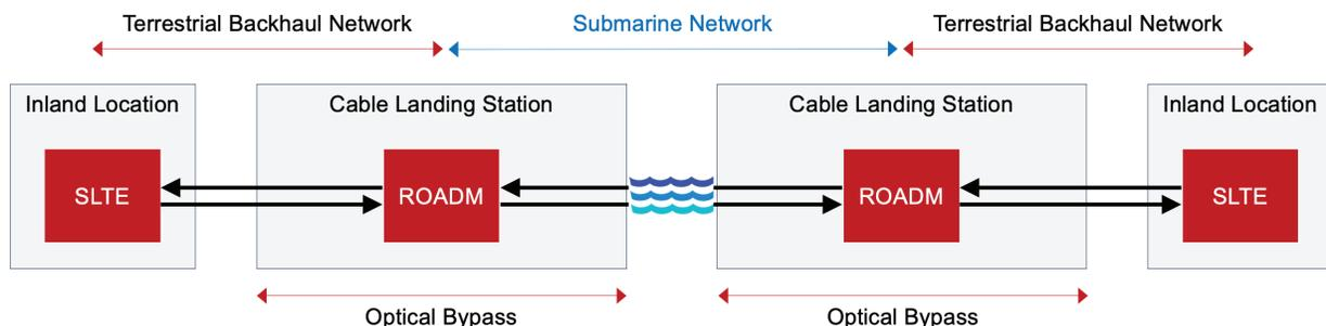
Figure 3: Simpler end-to-end network design via coherent optical transmission (GeoMesh Extreme).
