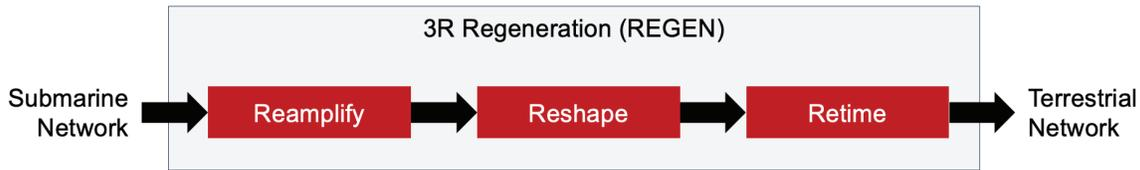
Figure 2: Traditional 3R (Reamplify, Reshape, Retime) regeneration stage.
