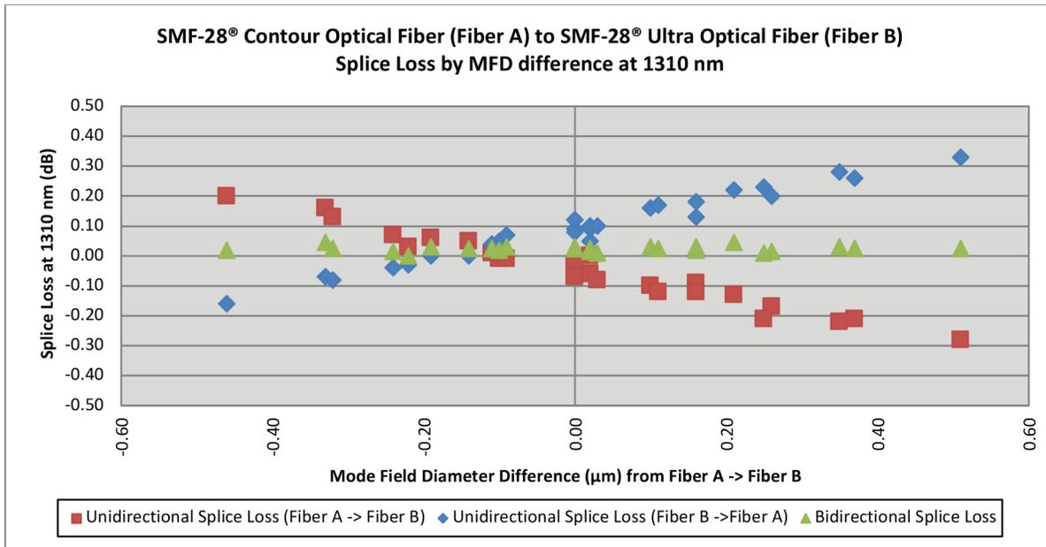
Figure 4: Unidirectional and Bidirectional Splice Loss.
