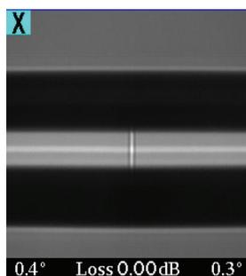
Figure 1. Homogeneous splice
