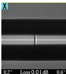
Figure 2. Heterogeneous splice
