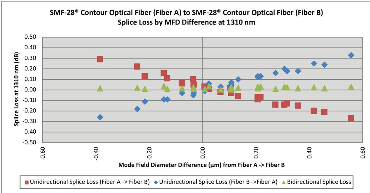
Figure 3. Unidirectional and Bidirectional Splice Loss.
