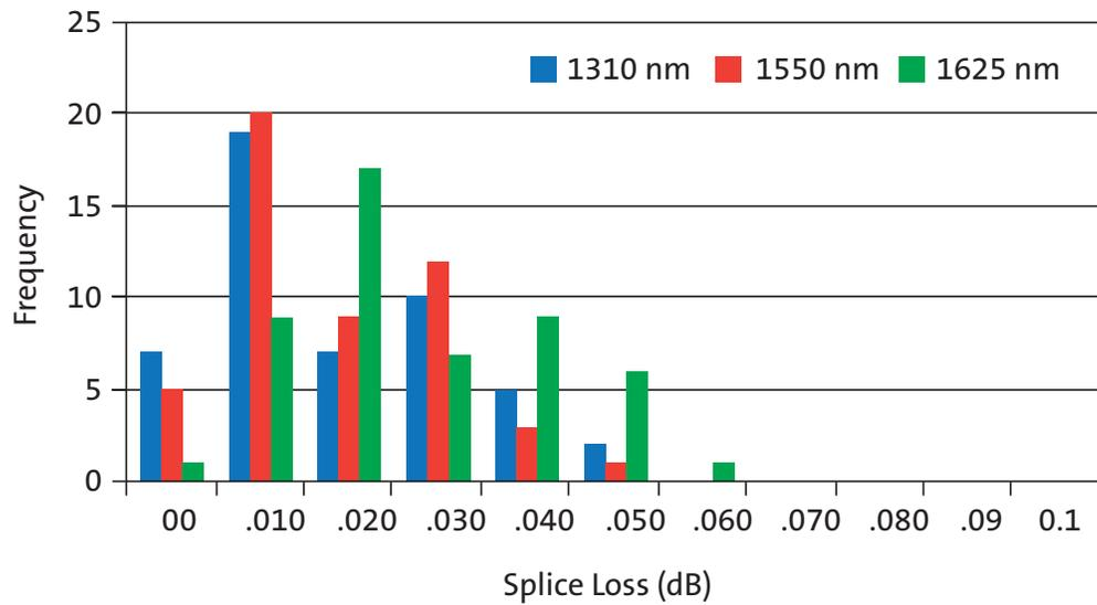
Figure 4. Representative splice loss of ITU-T.G652.D reduced diameter fiber spliced to itself.
