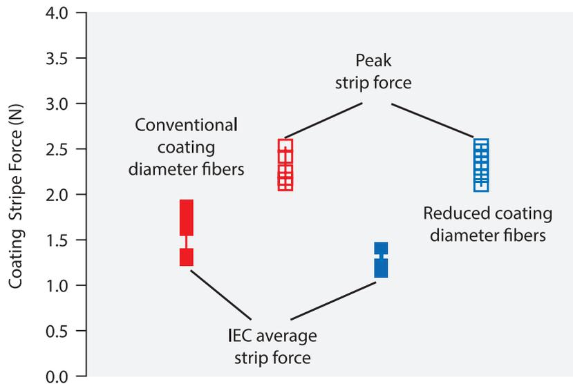
Figure 3. Comparison of coating stripe force: Conventional vs. reduced coating diameter fibers.
