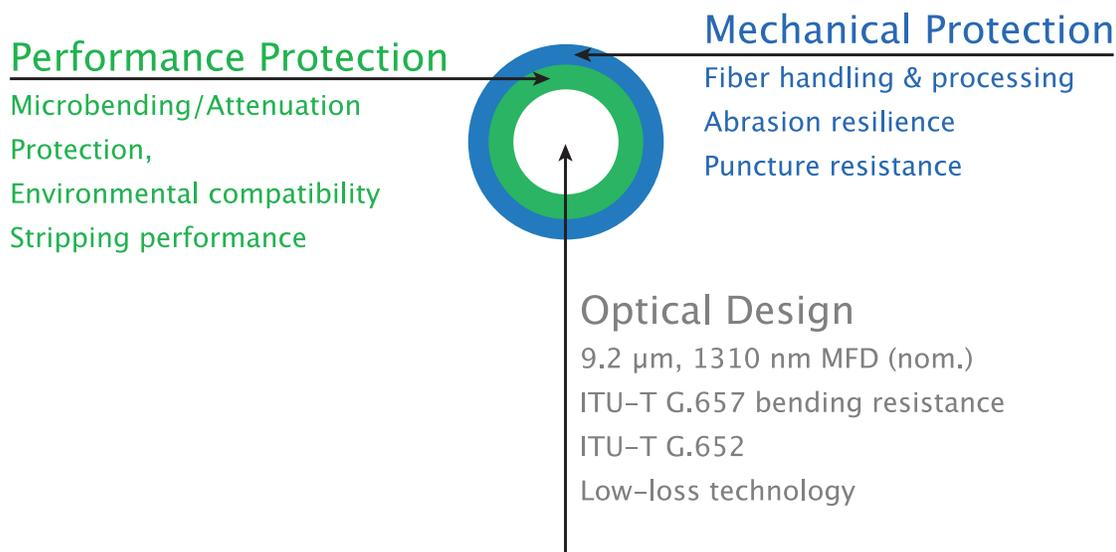
Figure 1. Two main principle functions of the dual-layer Corning CPC® protective coating and key design aspects of the central glass fiber.
