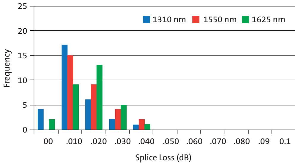
Figure 5. Representative splice loss of ITU-T.G652.D reduced diameter fiber spliced to convention diameter fiber.
