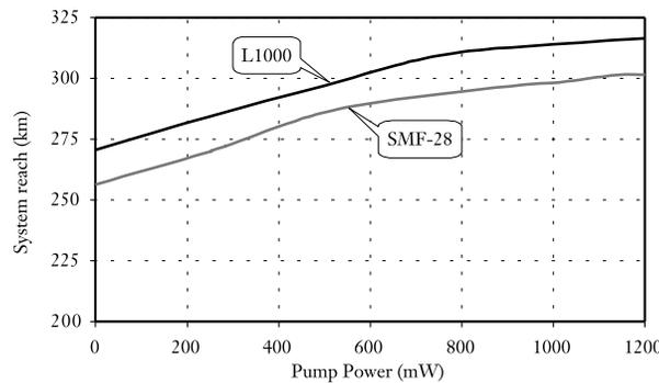
Figure 5. Maximum Span Loss for a BER of  $10^{-8}$  Versus Pump Power
