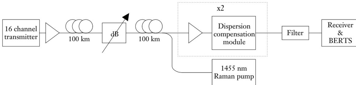
Figure 3. Experimental Configuration for Comparing Fibers with Different Effective Areas
