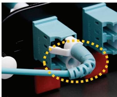
Figure 5. Pull connector as a result of entropy effect over time
