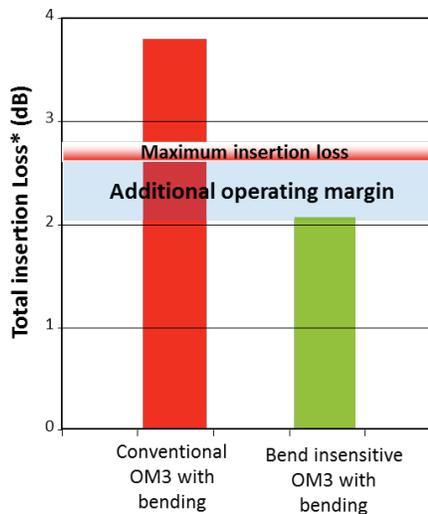
Figure 7. Bend insensitive OM3 fiber macrobend performance versus standard multimode OM3 fiber
