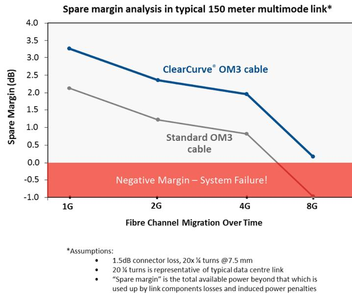
Figure 8. Spare margin analysis with Fiber Channel migration
