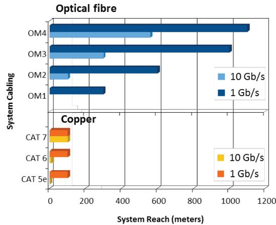
Figure 2. Optical systems networks allow higher data rates and system reach
