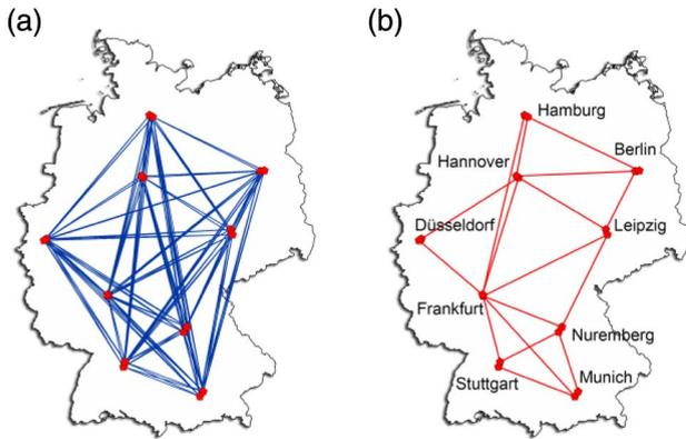
Fig. 1. Topology of (a) IP layer and (b) WDM layer.
