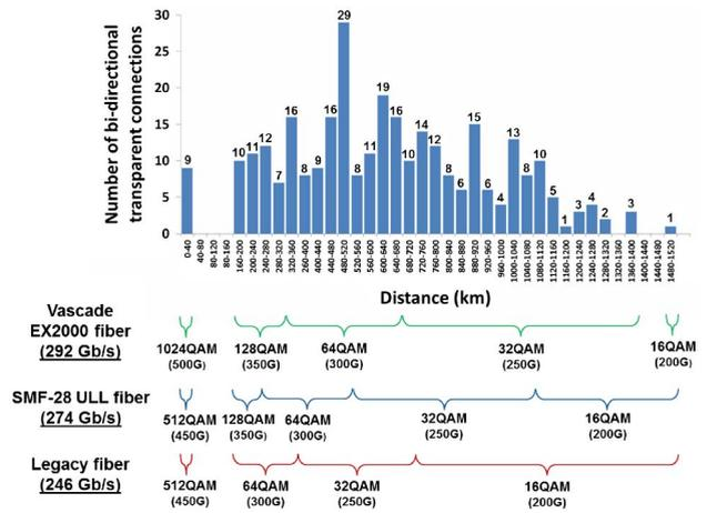
Fig. 4. Maximum achievable modulation density for each of the transparent connections in the histogram (40 km spans).
