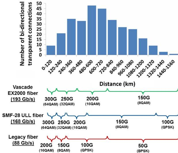
Fig. 5. Maximum achievable modulation density for each of the transparent connections in the histogram (120 km spans).
