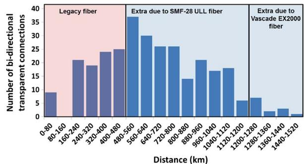
Fig. 2. Histogram of transparent connection lengths and coverage by fiber type at 200 Gb/s (PM-16QAM).
