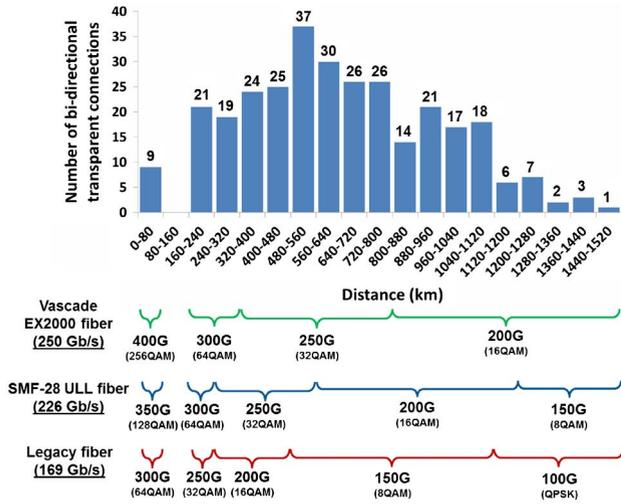
Fig. 3. Maximum achievable modulation density for each of the transparent connections in the histogram (80 km spans).
