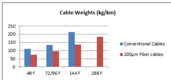
Figure 5. Cable Weight Comparison
