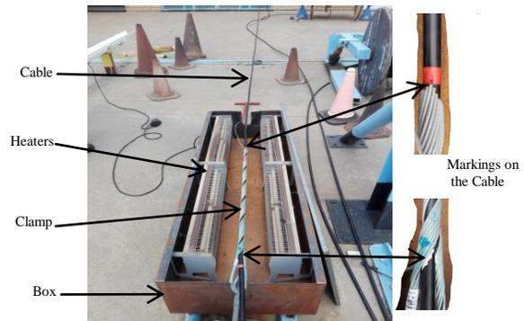
**Figure 9. Test Arrangement (“Hot-box”)**
