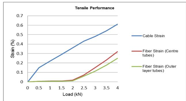
Figure 6. Cable Tensile Performance
