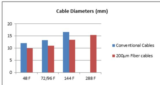
Figure 4. Cable Diameter Comparison
