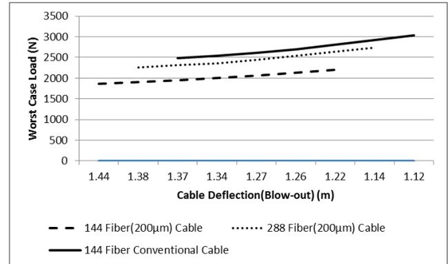
Figure 3. Worst Case Load vs Deflection (Blow-out)
