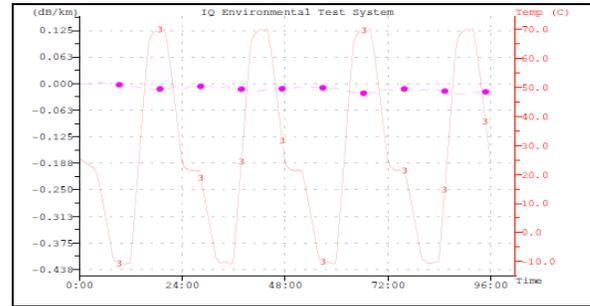
**Figure 8. Temperature Cycling at 1550 nm**
