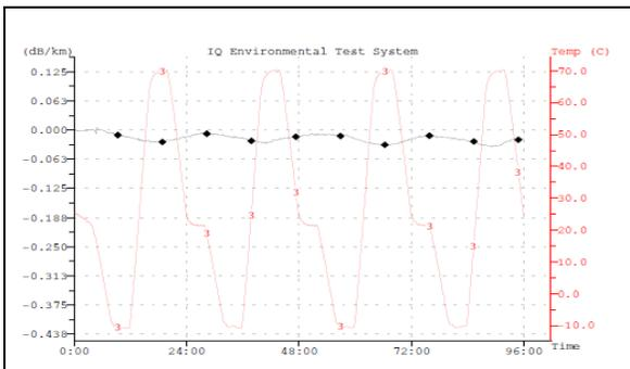
**Figure 7. Temperature Cycling at 1310 nm**
