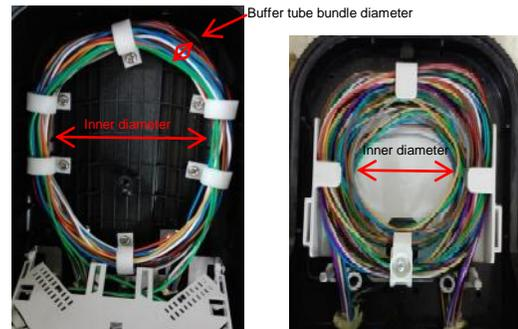
Figure 12. Inner Coil Diameter
