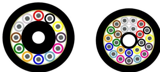
**Figure 1. ADSS Cables – 144 Fiber cable incorporating conventional ITU-T G.652.D fibers (left), and 288 Fiber cable incorporating G.657.A1 200 $\mu$ m fibers (right).**
