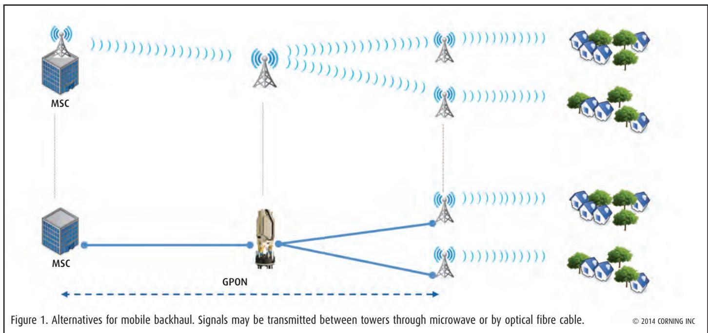
Figure 1. Alternatives for mobile backhaul. Signals may be transmitted between towers through microwave or by optical fibre cable. © 2014 CORNING INC
