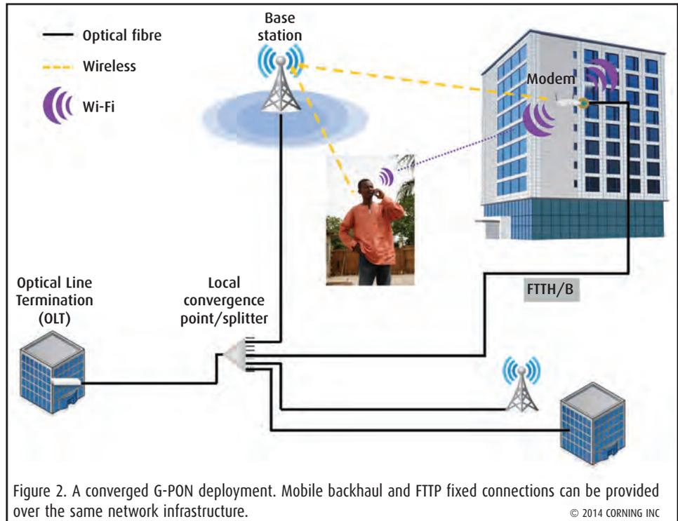
Figure 2. A converged G-PON deployment. Mobile backhaul and FTTP fixed connections can be provided over the same network infrastructure. © 2014 CORNING INC
