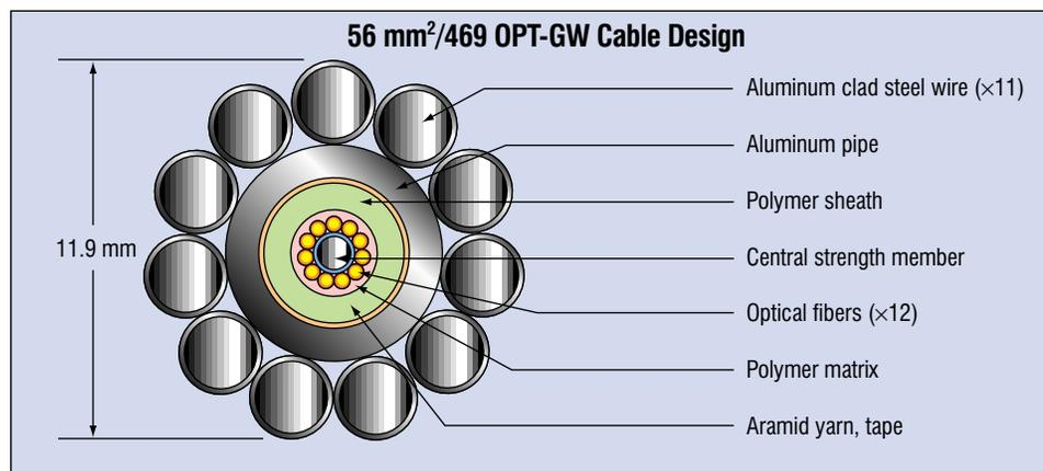
**Fig. 1.** This diagram depicts the 56 mm<sup>2</sup>/469 optical ground wire used for the test. The nomenclature 56 mm<sup>2</sup>/469 refers to the cross-sectional area of the stranded aluminum-clad steel wires (56 sq mm) and the outer diameter in thousandths of an inch (0.469 inch).
