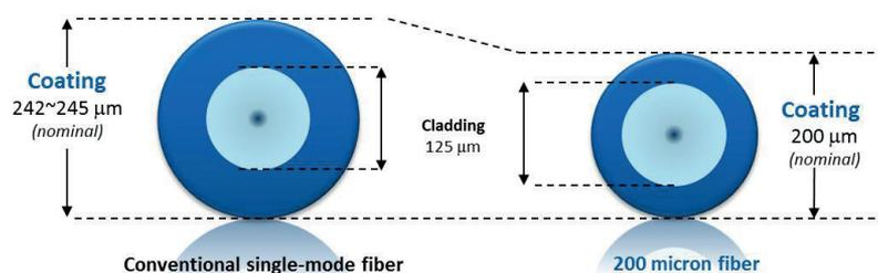
Cross sections of conventional and 200-micron fibres
