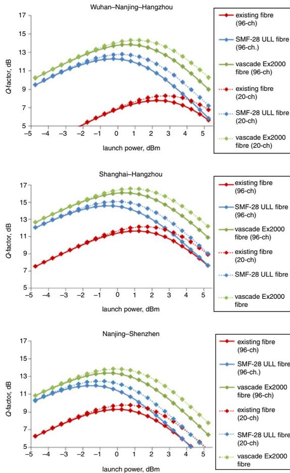
Fig. 3 200G 8QAM-based transmission comparison for different fibres
