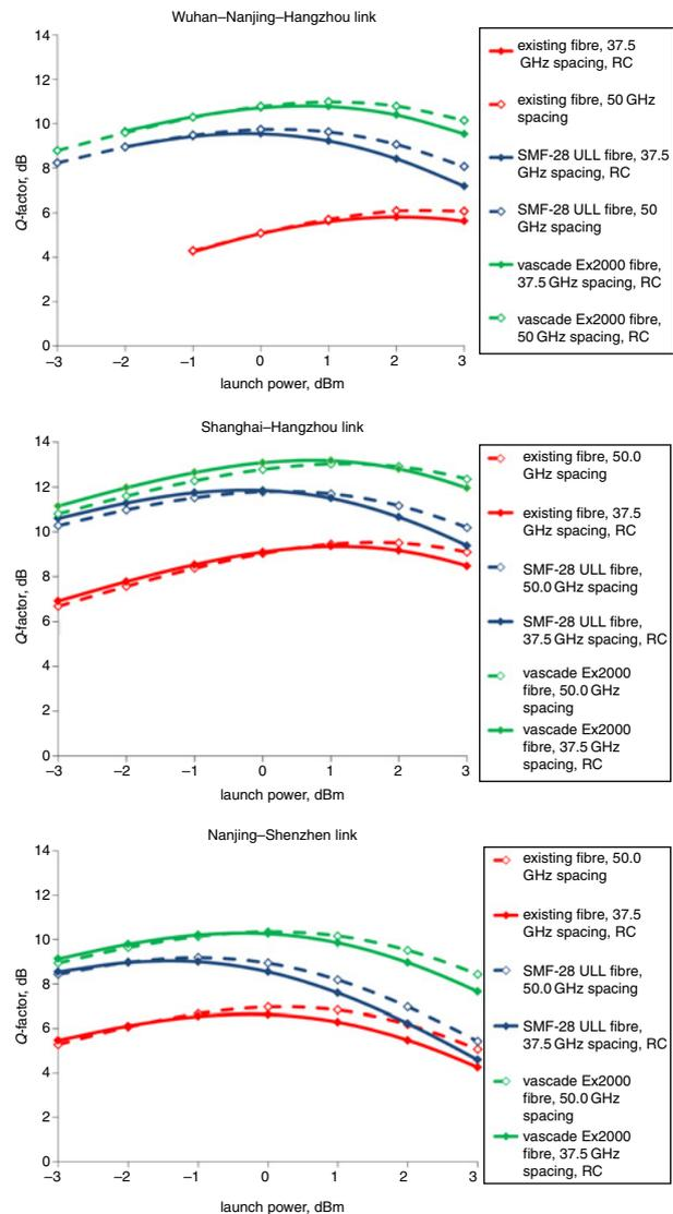
Fig. 2 200G 16QAM-based transmission comparison for different fibres
