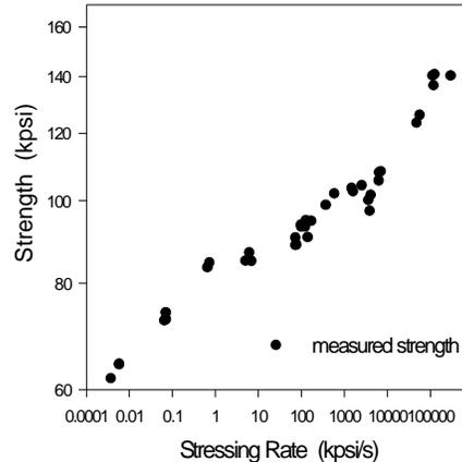
Figure 4. Middle strength values for a wide range of stressing rates in an ambient environment using draw-abraded fiber.
