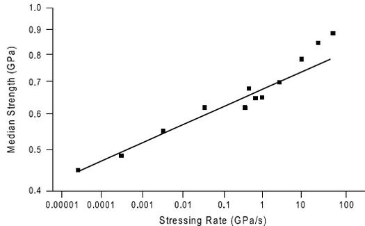
Figure 2. Dynamic fatigue plot showing curvature at high stressing rates from data in reference 4.
