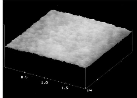
Figure 4: Auto-flattened and Plane-fit AFM scan of cable-aged fiber.
