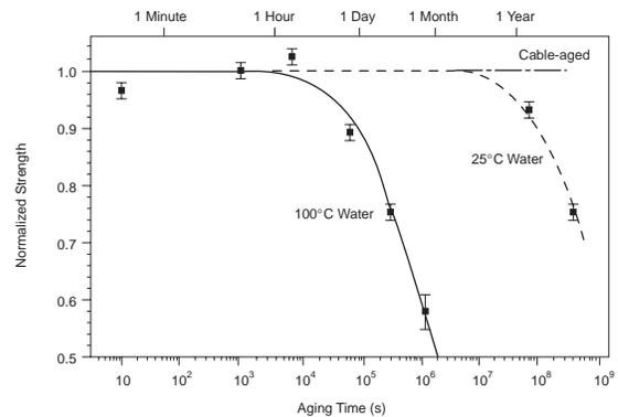
Figure 8: Comparison of strength degradation results obtained from fibers aged in the field and in laboratory<sup>5</sup> (liquid water).
