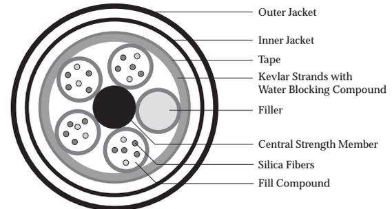
Figure 1: Schematic of the cable design.
