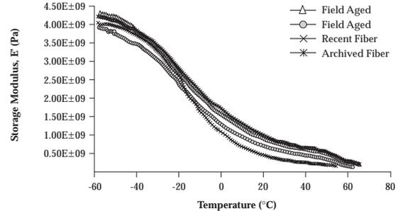
Figure 10: Coating Storage modulus ( $E'$ ) vs. temperature from DMA.
