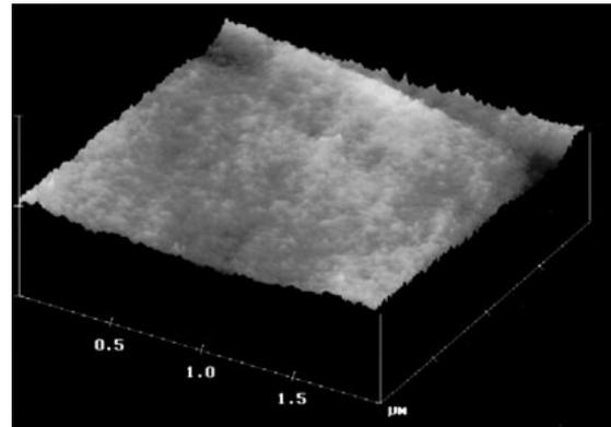
Figure 6: Auto-flattened and Plane-fit AFM scan of a recently manufactured fiber.
