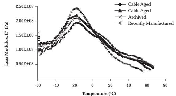
Figure 11: Coating Loss modulus ( $E''$ ) vs. temperature from DMA.
