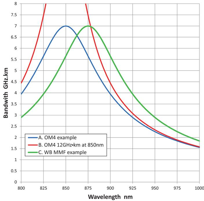
Figure 4. Bandwidth versus wavelength for three modeled fibers that illustrate the characteristics needed for a WB MMF.
