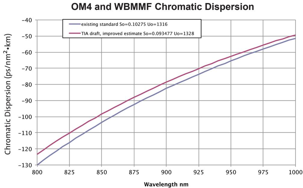
Figure 3. The Chromatic Dispersion penalty of a MM fiber is proportional to the dispersion and the spectral width of the transmitter. Improved estimates of chromatic dispersion in OM4 and WB MMF fibers enable longer distances at 850 nm with the same laser.
