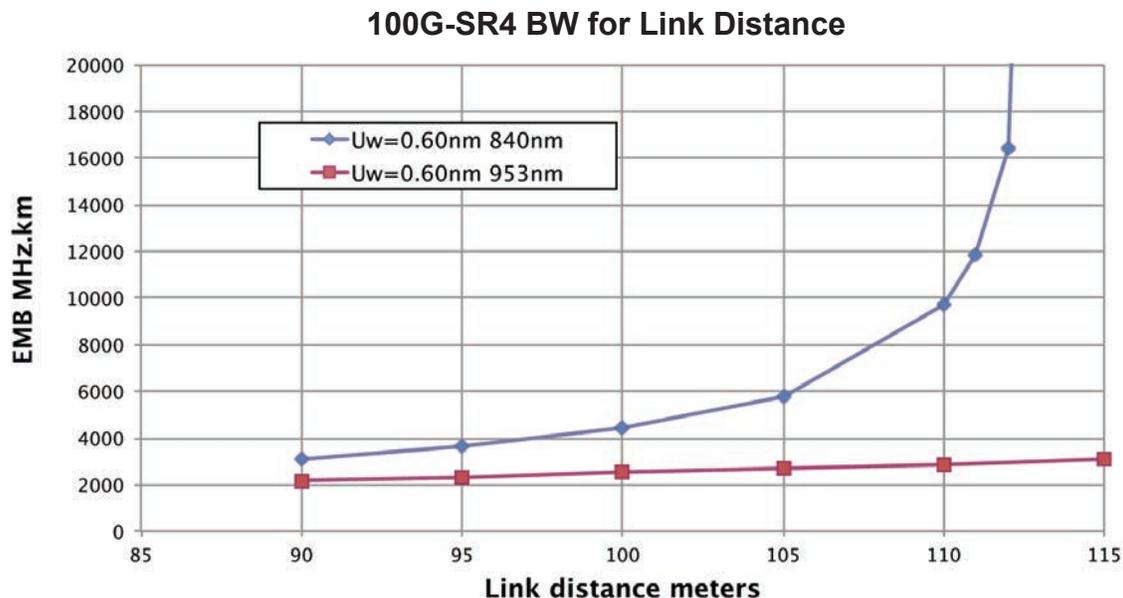
Figure 2. Required EMB versus link distance. The system reach at 840 nm is limited by the spectral width of the transceiver combined with chromatic dispersion, not by the bandwidth and intermodal dispersion. At 953 nm with reduced chromatic dispersion there is no limitation to distance in this range.
