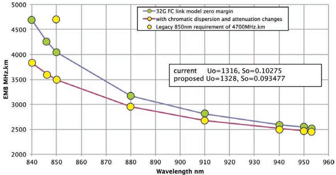
Figure 5. Required bandwidth versus wavelength in IEEE 100G-SR4 link model for two different chromatic dispersion parameters.
