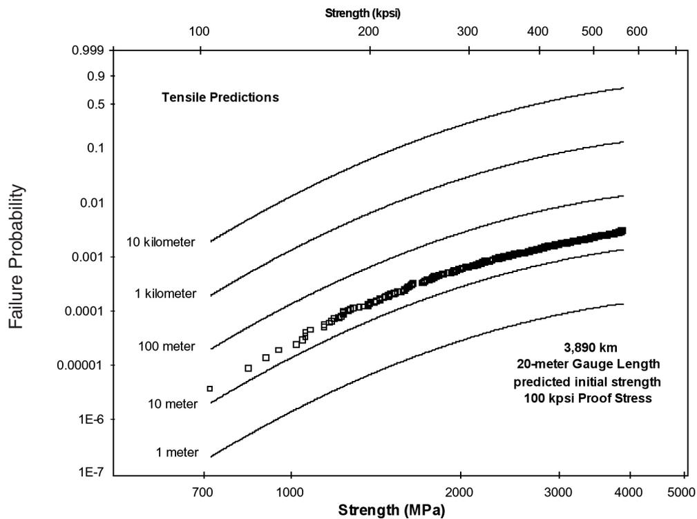
**Figure 2.** Strength of nearly 4000 km's of standard single-mode optical fiber. The lines represent predicted distributions for lengths other than 20 meters. Note that fatigue during strength testing has been accounted for. This distribution is ready to be incorporated into reliability models.
