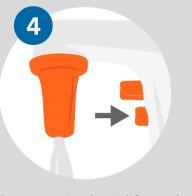
Dispense the excessive liquid from the pipet until the meniscus of the liquid aligns exactly with the required volume mark on the pipet.
