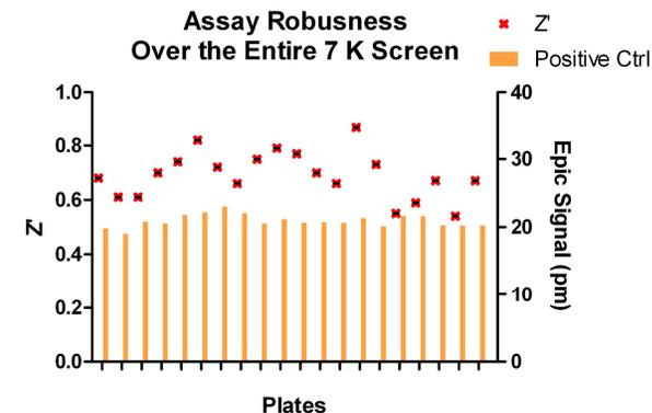
**Assay Robustness:** Over the 20 Epic microplates used for the 7 K screen, the positive control signal of 21 pm and the robustness, the  $Z'$  factor, is  $\sim 0.7$ .
