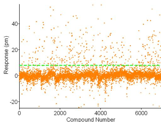
A majority of the compounds give a signal very close to zero. The threshold (**5MAD**) is represented by the green dashed line. It is clearly seen that the hits are well distributed along the 20 microplates of the screen, indicating that the hit distribution is not biased.
