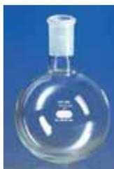
**4320C PYREX Flask, Boiling, Round Bottom, Short Neck, Heavy Wall, ⚗ Joint**
