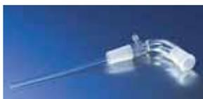
**8945 PYREX Adapter, Connecting, 105° Angle, Two-way, Vacuum Suction Tube, 10mm O.D., 24/40 Joints**
