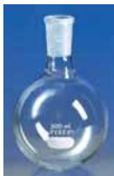
**4320A PYREX Flask, Boiling, Round Bottom, Short Neck, ⚗ Joint**
