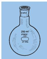
**4320B PYREX Flask, Boiling, Round Bottom, Short Neck, ⚗ Joint**
