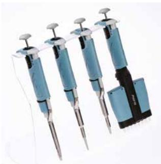
Axygen Axypet single- and 8-channel pipettors
