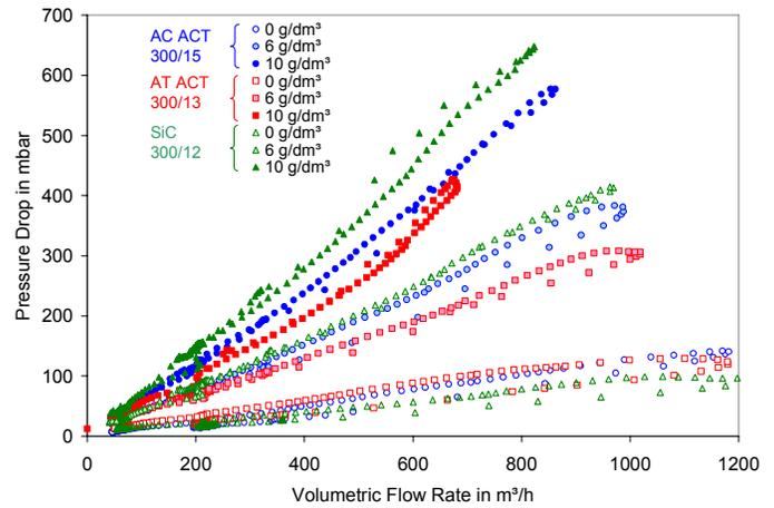
Figure 2: Pressure drop measured on an engine dynamometer, for reference there is 300 cpsi segmented SiC filter, advanced cordierite with ACT and aluminum titanate with ACT at 0, 6 and 10 g/liter soot
