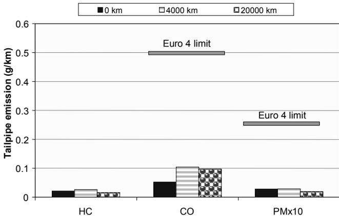
Figure 8: MVEG-B test cycle emissions for Pt/Pd catalyzed aluminum titanate filter-only on a 2.0 liter Vehicle B over 20,000 km of AMA cycle ageing
