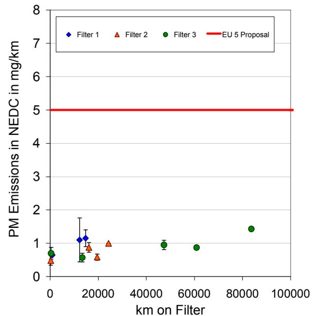
Figure 6: PM emissions over the MVEG-B test cycle for a DOC and catalyzed cordierite filter fitted on a European vehicle with a 3.0 liter diesel engine
