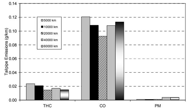
Figure 5: Tailpipe emissions over the MVEG-B test cycle from a 2.2 liter vehicle originally equipped with a fuel additive system and bare SiC filter, but retrofitted with a single unit catalyzed advanced cordierite filter
