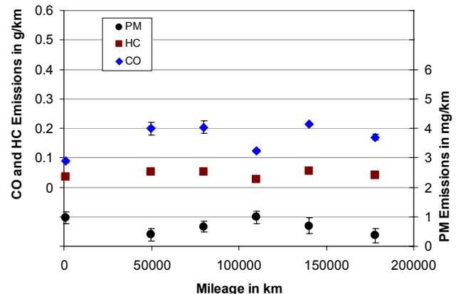
Figure 10: MVEG-B test cycle emissions for Pt/Pd catalyzed aluminum titanate filter-only on a 2.0 liter Vehicle D over >150,000 km of real-world driving
