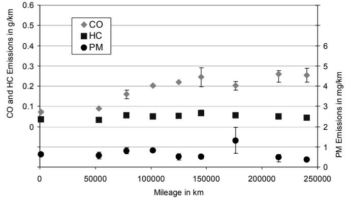
Figure 9: MVEG-B test cycle emissions for catalyzed aluminum titanate filter-only on a 2.0 liter Vehicle C over 240,000 km of real-world driving
