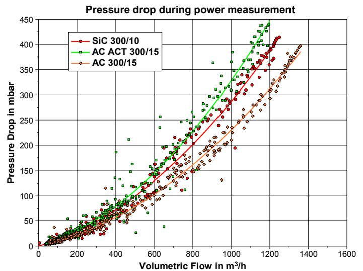
Figure 3: Pressure drop measurements in the “nearly clean” state (<40 km on new filter), as tested on a 3.0 liter diesel vehicle. OEM reference SiC filter and AC filter had 4.6 liter and 4.1 liter volume, respectively.
