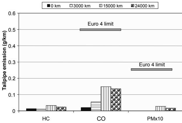
Figure 7: MVEG-B test cycle emissions for catalyzed aluminum titanate filter-only on a 1.9 liter Vehicle A over 24,000 km of AMA cycle ageing
