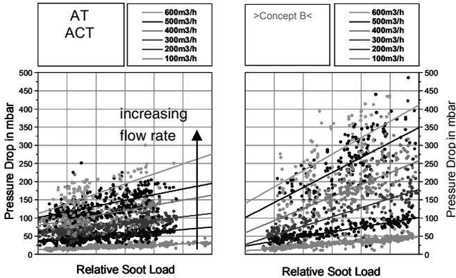
Figure 4: Pressure drop measurements as a function of soot loading at various flow rates for an aluminum titanate filter with ACT and “concept B” an OEM reference 300 cpsi segmented SiC filter – high porosity, as tested on a 2.0 liter diesel vehicle. Both filters had a 3.0 liter volume [3]
