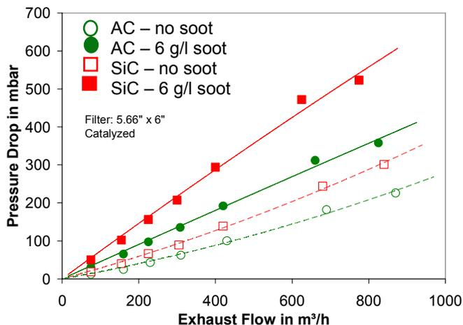
Figure 1: Filter pressure drop as tested on engine dynamometer - reference 200 cpsi segmented SiC and advanced cordierite with ACT at 0 g/liter and at ~ 6.5 g/liter soot (at increasing speed and load to increase flow rate)
