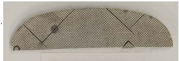
Figure 11. Filter sample E outlet end photo after survivability test.
