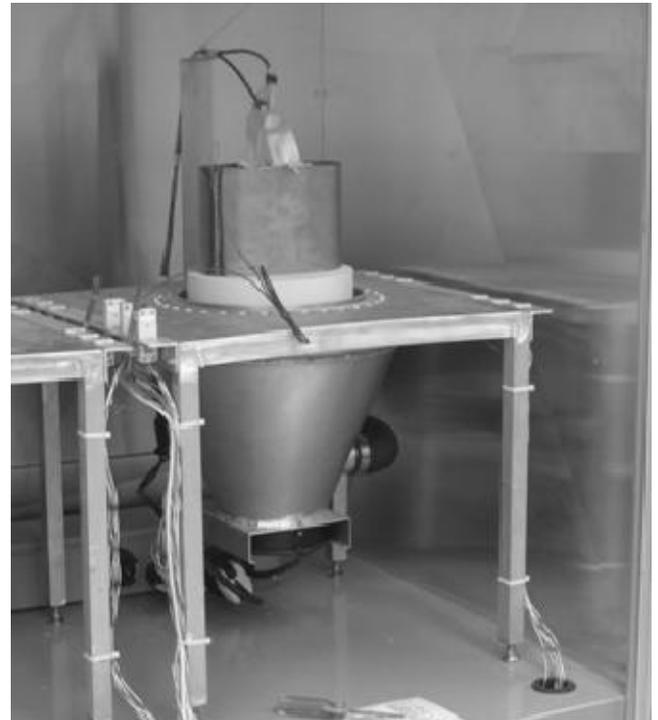
**Figure 12: Example of Aluminum Titanate Oval on RTE Test Stand**
