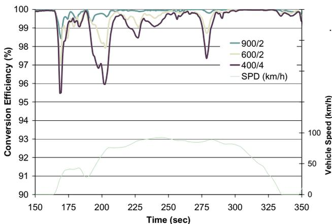
Figure 8: Hydrocarbon Conversion Efficiency at Hill 2 in Bag 1
