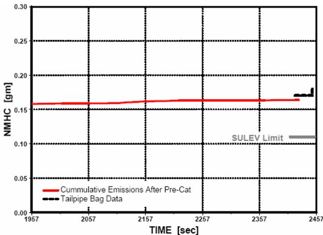
Figure 14: Phase 3 HC Emissions for 900/2 - accumulated, bag and regulation
