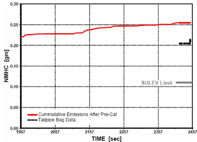
Figure 10: Phase 3 Hydrocarbon Emissions for 400/4 - accumulated, bag and regulation
