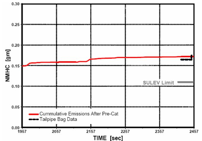
Figure 12: Phase 3 HC Emissions for 600/2 - accumulated, bag and regulation
