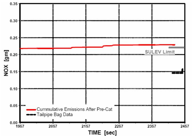
Figure 15: Phase 3 NOx Emissions for 900/2 - accumulated, bag and regulation
