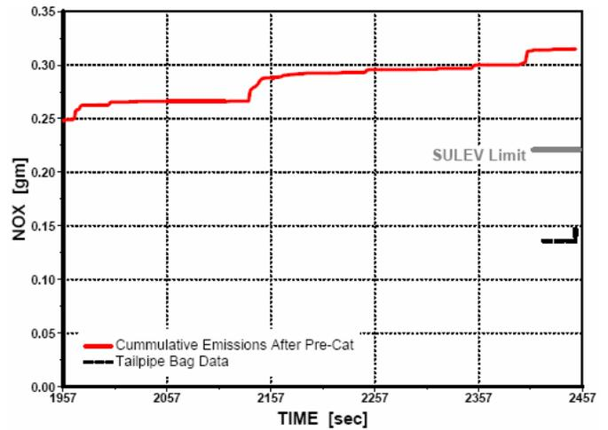
Figure 11: Phase 3 NOx Emissions for 400/4 - accumulated, bag and regulation
