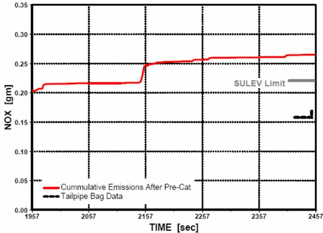
Figure 13: Phase 3 NOx Emissions for 600/2 - accumulated, bag and regulation
