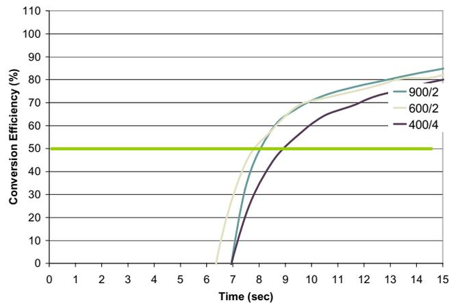
Figure 9: HC Conversion Efficiency in first 15 seconds
