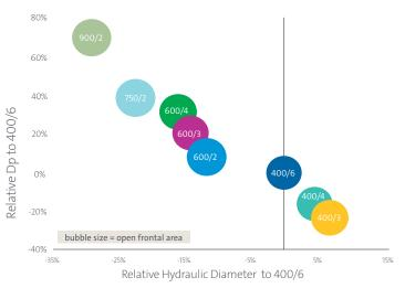
\*Parts tested at size 105.7 x 76 mm; bp @ 200kg/h & 800C
