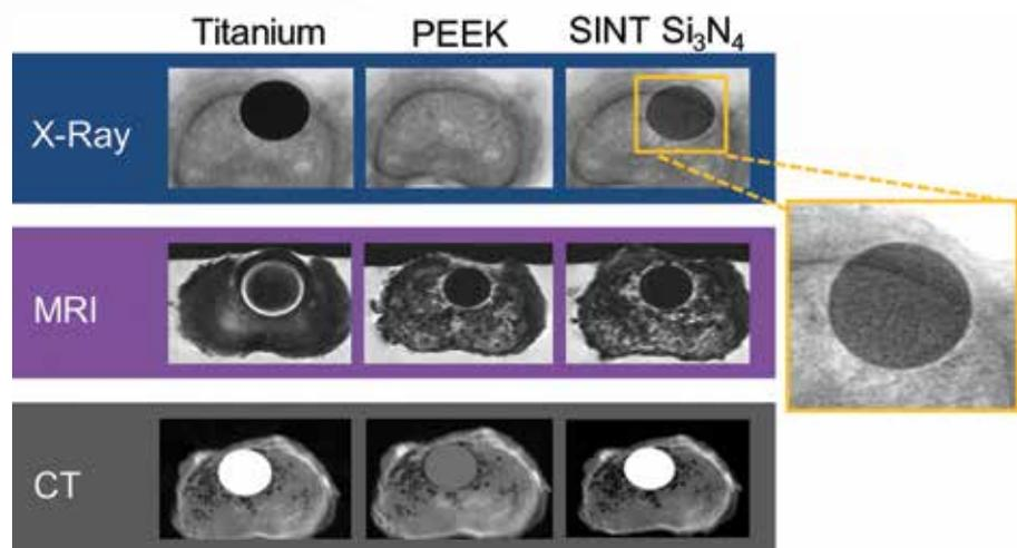
**Figure 1. Comparison of implant visibility during medical imaging.**
