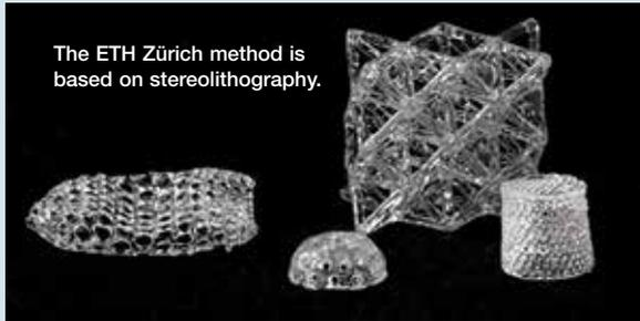
The ETH Zürich method is based on stereolithography.
