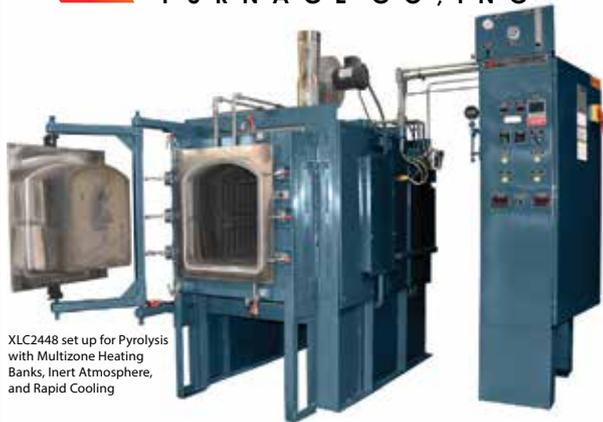
XLC2448 set up for Pyrolysis with Multizone Heating Banks, Inert Atmosphere, and Rapid Cooling
