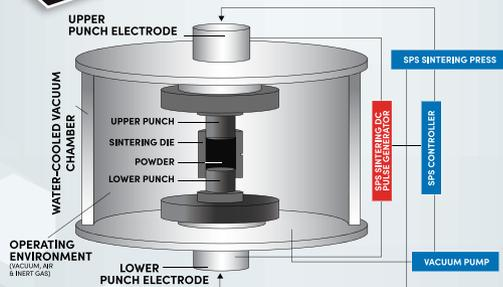
Sinter without any Binders! / Controlled Densification up 99-100%
