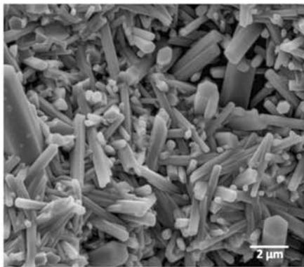
Figure 3. Surface microstructure of bioactive Si<sub>3</sub>N<sub>4</sub>.
