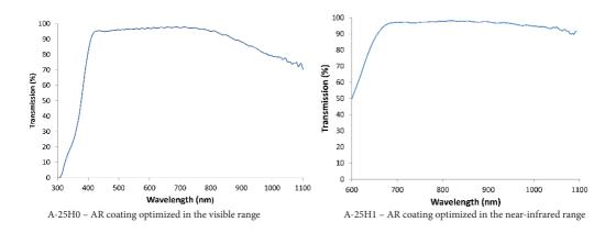
With an anti-reflective coating optimized in the near infrared, the transmission curve flattens from 700nm to 1100 nm.
