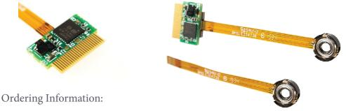
A-PE-25H0-33: Packaged A-25H0 with electronics and FPC-A-33
