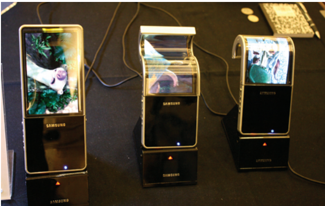
FLEXIBLE OLED DISPLAYS COULD SIGNAL THE END OF THE USE OF RIGID SHEETS OF GLASS TO ENCAPSULATE A SCREEN PHOTO: OLED-DISPLAY.NET
