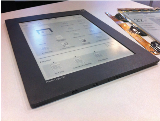
THE PLASTIC LOGIC 100 USES A FLEXIBLE BACKPLANE TECHNOLOGY FOR ITS E-READER DISPLAY PHOTO: INTERTECHPIRA
